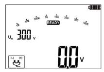
After inserting WS-04 into the socket, the screen displays a message indicating the detection of the adapter.
