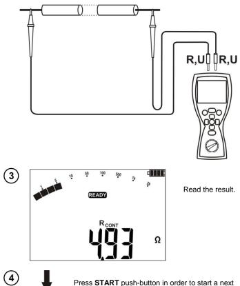
Press **START** push-button in order to start a next measurement without disconnecting test leads from the object.
