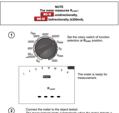
The measurement starts automatically when the meter detects a resistance within the measurement range. The measurement may be also triggered manually by pressing **START** push-button.
