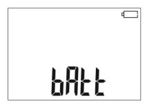
Batteries / rechargeable batteries fully discharged. The meter switches off automatically.
